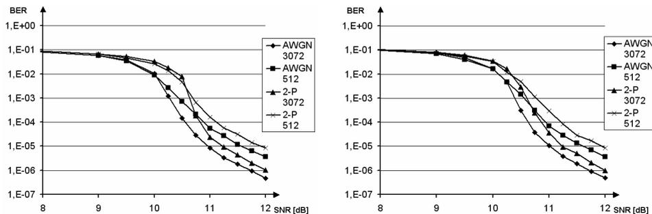
Fig. 3.3. Comparison of results for the MAP algorithm (left) and for the SOVA algorithm (right)
