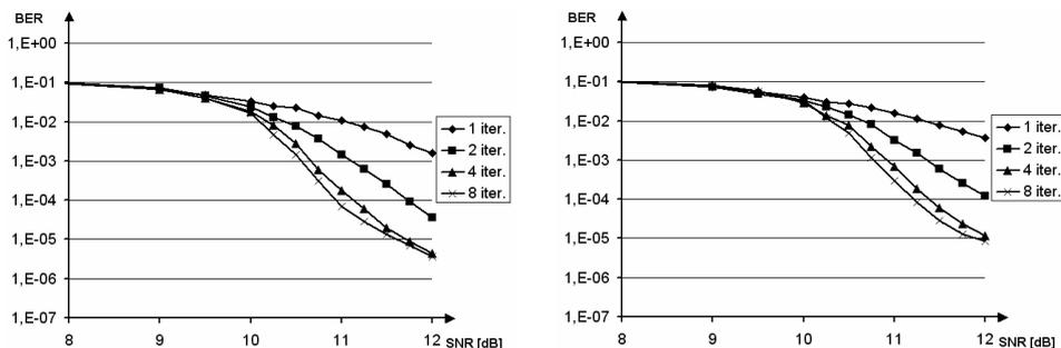
Fig. 3.2. Results for the SOVA algorithm,  $N = 512$ , AWGN channel (left) and two-path channel (right)
