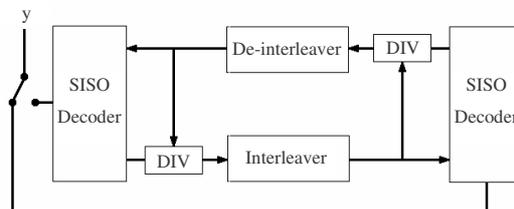
Fig. 1.2. Block diagram of parallel TTCM decoder [4]
