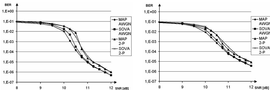
Fig. 3.4. Comparison of results for interleaver size  $N = 3072$  (left) and for  $N = 512$  (right)
