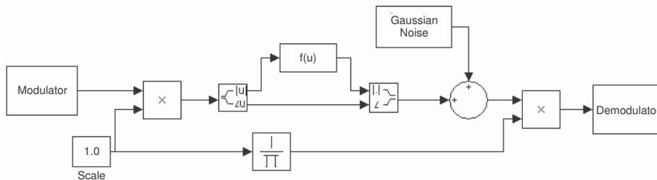
Fig. 2.1. Block diagram of Simulink simulation model
