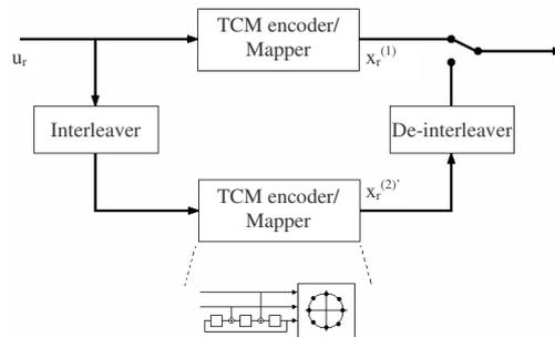
Fig. 1.1. Block diagram of parallel TTCM encoder with 8PSK encoders [4]
